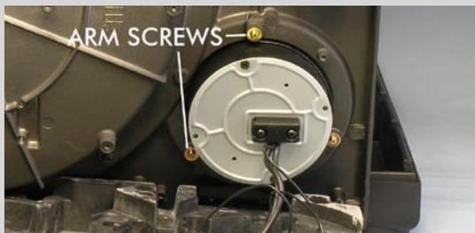
Remove the 3 screws holding on the Technics arm and then the screw which fastens the black earth lead. The arm can now be removed. You will need to re-earth this connection and ensure that it makes electrical contact with the arm earth wire or base of the arm if it is metal (wedging the strands of wire underneath the arm base nut is the easiest method of doing this.
