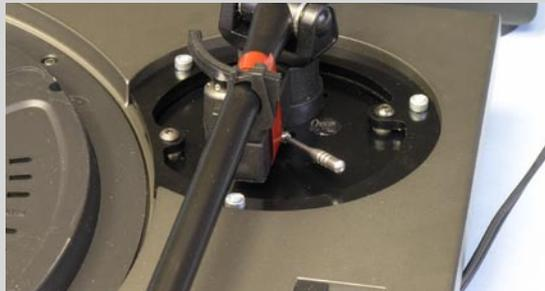
Thread the 3 off nylock nuts with washers onto the underside of the bolts just fitted to hold on the new armboard. Tighten nuts but not too hard or you may crush the mounts on the deck.
