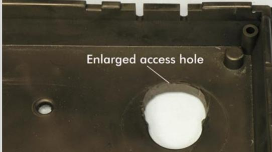
Enlarge the hole for the arm leads in the outer moulding. This enables you to access the large nut on the underside of the armboard should you ever need to adjust it. Use a Stanley knife blade to cut the hole.
