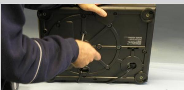
Unscrew the 4 feet and then ALL 21 or so cross-head screws on the underside of the deck which hold on the base cover.
