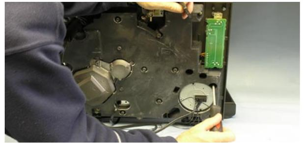
Remove the 6 or so brass coloured cross head screws from the underside of the inner base moulding. Mark the positions of these screws for re-insertion as it is easy to forget the positions and get them confused with other holes. Do not remove the 4 screws that hold on the hinges.
