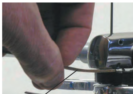
CORK STRIP INSERTED ON LEFT SIDE IN 1.5MM GAP BETWEEN YOKE AND TURRET PLATE
