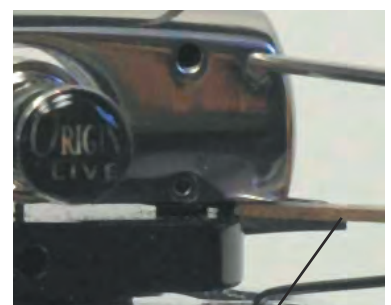
CORK STRIP INSERTED ON RIGHT SIDE IN 1.5MM GAP BETWEEN YOKE AND TURRET PLATE
