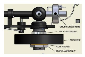
You now need to adjust the <u>height</u> of the arm base to its correct position using the threaded VTA adjuster ring (as shown above).
