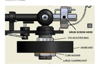
Insert the arm through the arm-board hole and fit the cork washer underneath followed by the large clamping nut. Turn the nut to finger tight as hard as you can (see above diagram).
