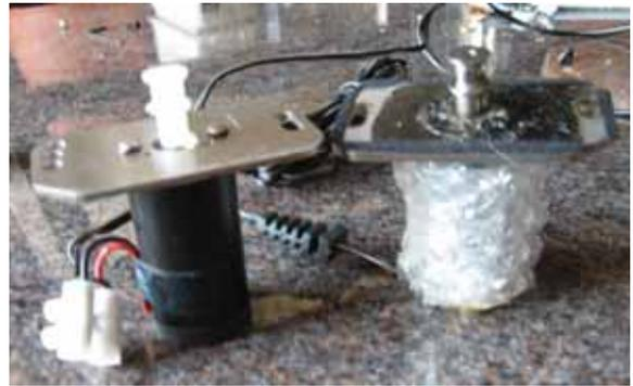
*The new OL DC 200 motor left, with the old (sound proofed) unit on the right.*
