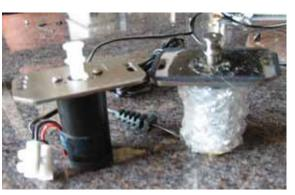
The new OL DC 200 motor left, with the old (sound proofed) unit on the right.
