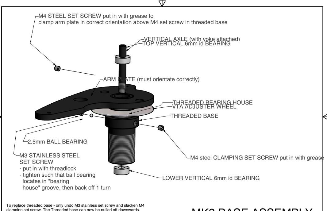
To replace threaded base - only undo M3 stainless set screw and slacken M4 clamping set screw. The Threaded base can now be pulled off downwards. Replacement is a reversal of the removal process only remember to ensure the 2.5mm ball bearing is inserted and read drawing note about backing off 1 turn.
