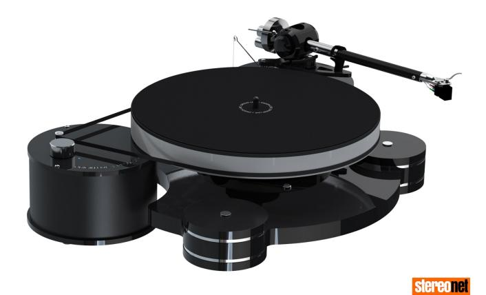
The low friction main bearing runs in an oil bath for smooth results. With the belt removed, the time taken for the platter to stop turning from 33.3rpm was 1 minute, 42 seconds. That's really impressive. By way of comparison, despite its massive 12kg platter, Acoustic Solid's MPX turntable took 1 minute 20 seconds, and my reference Musical Fidelity MF-1 lasted less than 30.
