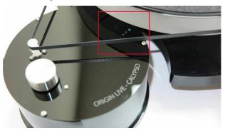
The sensor reads the silver strip on the underside of the platter (see below). This strip must never be removed or the speed will not be correct.
