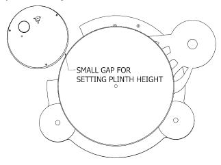
Set plinth height using the adjustable feet, to give the platter 4 to 7mm clearance between the top of the motor pod screws and the underside of the platter as shown below.
