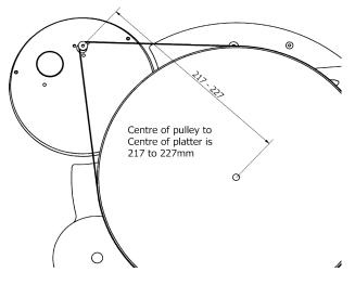
Fit the belt over the platter first and then pull it over the motor pulley taking care not to twist it. To set belt tension, simply move the pod.
