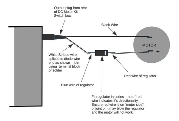
NOTE for production in Origin Live only: Middle leg of 1.2V regulator is blue wire Outer 2 legs are red wire Wrap in regulator in heat shrink
