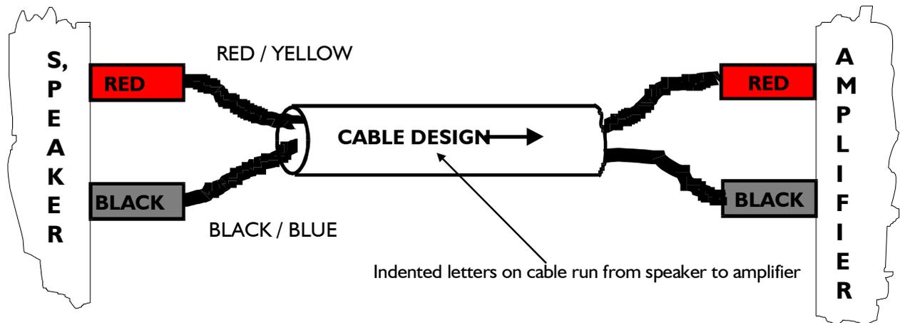
cables away from mains cable (i.e. plug sockets and leads for equipment). Avoid coiling wires from different channels together.
