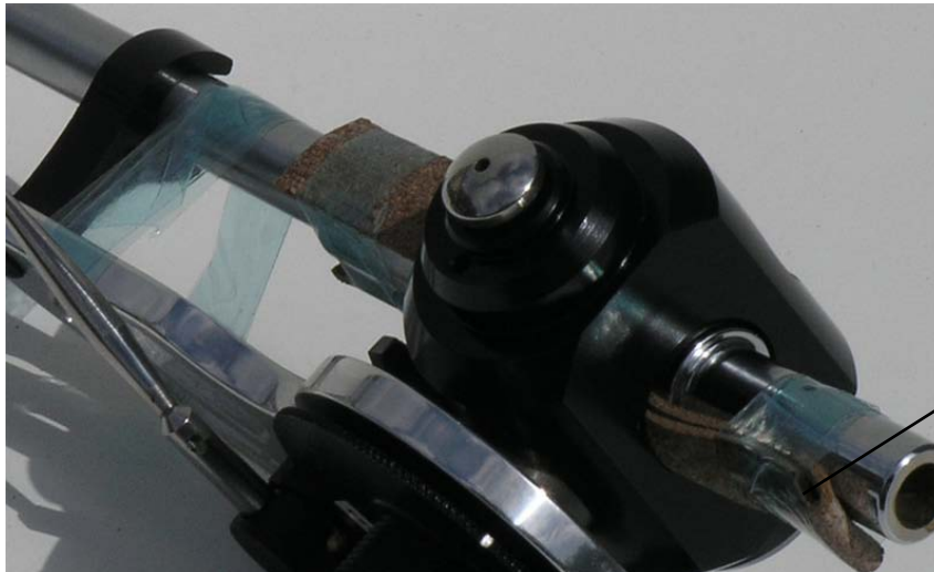
CORK PACKING PEICE WEDGING ARM TUBE TIGHTLY INTO TOP OF YOKE AND TAPED ON
