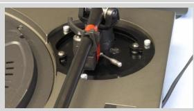
Thread the 3 off nylock nuts with washers onto the underside of the bolts just fitted to hold on the new armboard. Tighten nuts but not too hard or you may crush the mounts on the deck.
