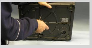
Unscrew the 4 feet and then ALL 21 or so crosshead screws on the underside of the deck which hold on the base cover.
