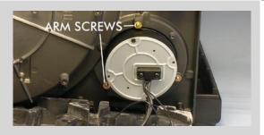
Remove the 3 screws holding on the Technics arm and then the screw which fastens the black earth lead. The arm can now be removed. You will need to re-earth this connection and ensure that it makes electrical contact with the arm earth wire or base of the arm <u>if it is metal</u> (wedging the strands of wire underneath the arm base nut is the easiest method of doing this.
