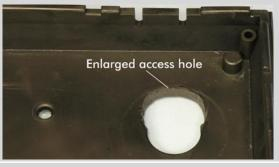
Enlarge the hole for the arm leads in the outer moulding. This enables you to access the large nut on the underside of the armboard should you ever need to adjust it. Use a Stanley knife blade to cut the hole.
