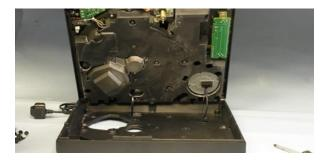
Remove the outer base cover by pulling it off.
