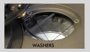
Place 3 washers over the holes in the arm well that the armboard will be fitted to.
