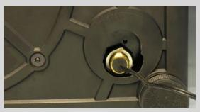
Refit the inner moulding using the 6 screws. Ensure that the arm cable goes through the hole in the arm base and that the mains lead is clear etc to enable the inner base to fit down properly.
