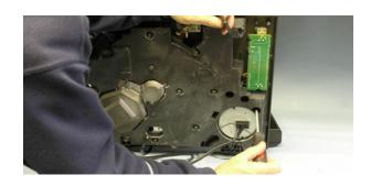
Remove the 6 or so brass coloured cross head screws from the underside of the inner base moulding. Mark the positions of these screws for re-insertion as it is easy to forget the positions and get them confused with other holes. Do not remove the 4 screws that hold on the hinges.
