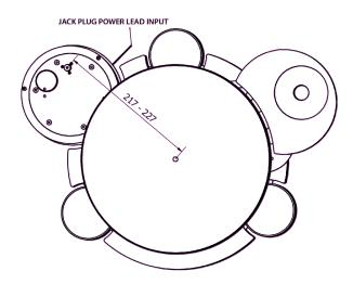
Fit the belt over the platter first and then pull it over the motor pulley taking care not to twist it.
