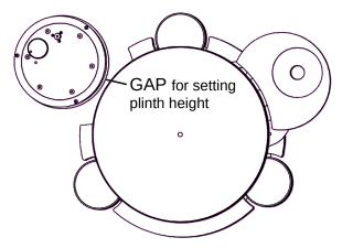
Set the plinth height by rotating the 3 adjustable feet. It helps to lift the deck slightly for access to each foot in turn.to set the plinth height correctly, position the motor pod just clear of the platter as shown below. Correct height description
